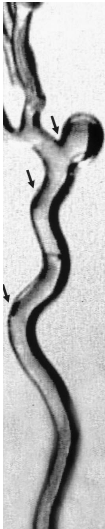
FIG 1. Elastic anatomic model with physiological curves of internal carotid artery and with aneurysm located on supraclinoid segment. Arrows show increased flow intensity at these points, caused by centrifugal effect of fluid.
