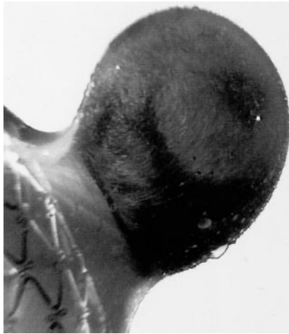
FIG 2. Lateral cross-section view of aneurysm model with implanted stent across neck.
